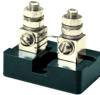
Our precision 50mV and 100mV base-mounted current shunts are designed for measuring dc currents from 5A to 1200A. These precision shunts ( $\pm 0.25\%$  accuracy) connect directly to the DATEL DCA5 Series of dc ammeters. Installation is straightforward: simply connect the load circuit to the shunt's threaded studs and the shunt's mV Kelvin-outputs to the digital ammeter's input terminals.
