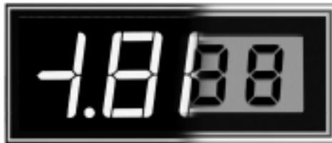
Backlit LCD displays should be used if the meter is to be operated in both high and low-light conditions. DATEL uses reliable, long-life LED's as the light source in all of our backlit LCD meters. A "B" suffix added to the end of the DATEL model number specifies a backlit model.
